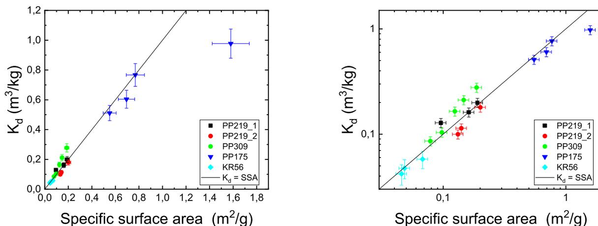
**Fig. 6.** The distribution coefficients ( $K_d$ ,  $m^3/kg$ ) of Cs for studied rocks (PP219\_1, PP219\_2, PP309, PP175 and KR56) as a function of specific surface area (SSA,  $m^2/g$ ). The results presented in linear (left) and logarithmic scale (right). Solid line shows trend line  $K_d$  ( $m^3/kg$ ) = SSA ( $m^2/g$ ) and correlation coefficient of  $K_d$  of Cs and SSA is 0.95. The different data points for each rock sample correspond to different grain sizes.
