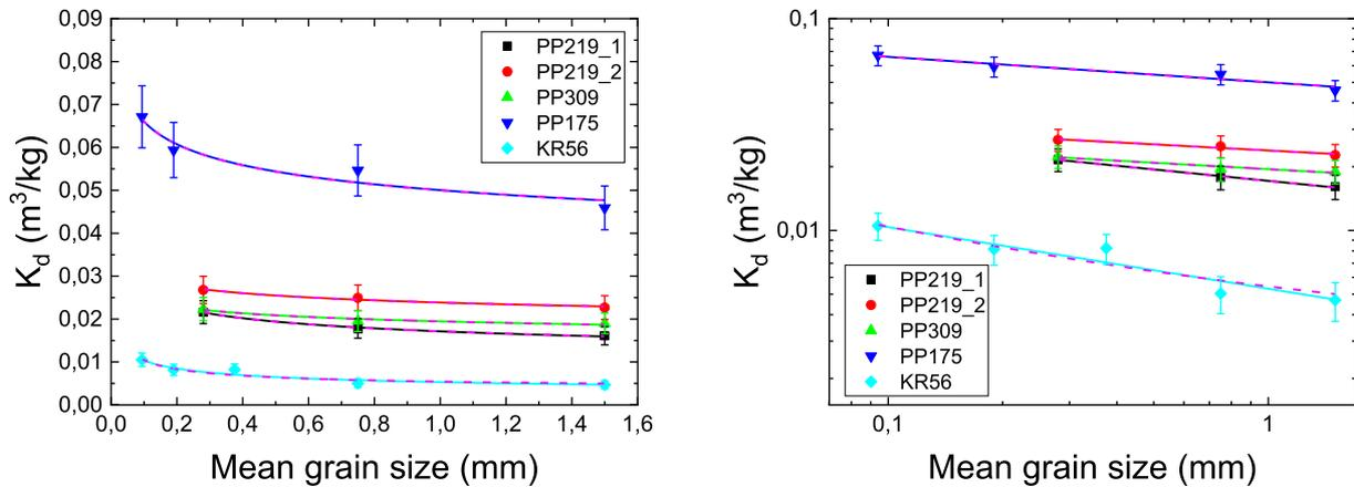
**Fig. 4.** The distribution coefficient of Sr on PP219\_1, PP219\_2, PP309, PP175 and KR56 as a function of mean grain size. The graph is shown on a linear scale (left) and on a logarithmic scale (right). Solid lines show fits by Eq. (8) and dashed lines by Eq. (9). The experiments have been performed in Sr concentration of  $1 \times 10^{-6}$  M. The error bars are standard deviations of the means of three parallel measurements.
