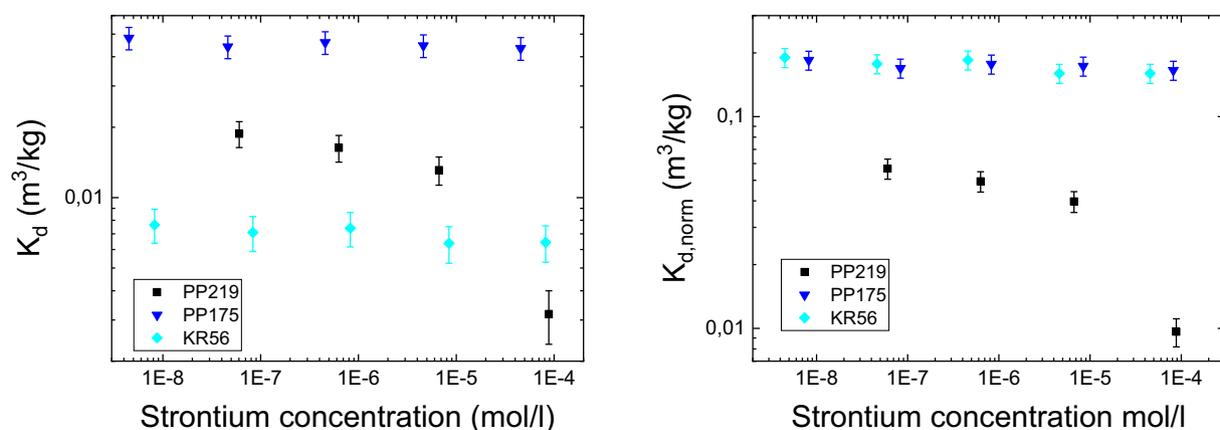
Fig. 2. The distribution coefficient ( $K_d$ , m<sup>3</sup>/kg) of Sr on crushed rocks a function of equilibrium Sr/kg concentration. The measured distribution coefficients (left) and normalized coefficients according to their mica content (right) are shown. The error bars are standard deviations of the means of three parallel measurements.
