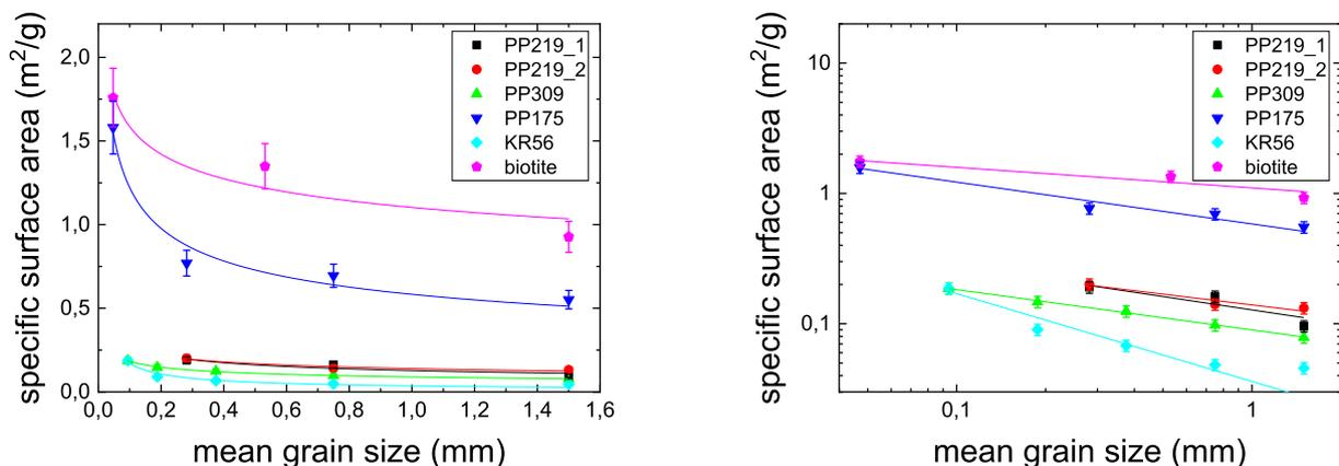
**Fig. 5.** The specific surface areas (m<sup>2</sup>/g) of studied rocks (PP219\_1, PP219\_2, PP309, PP175 and KR56) and biotite as a function of grain size. The results presented in linear (left) and logarithmic scale (right) and solid lines show fits by Eq. (8).
