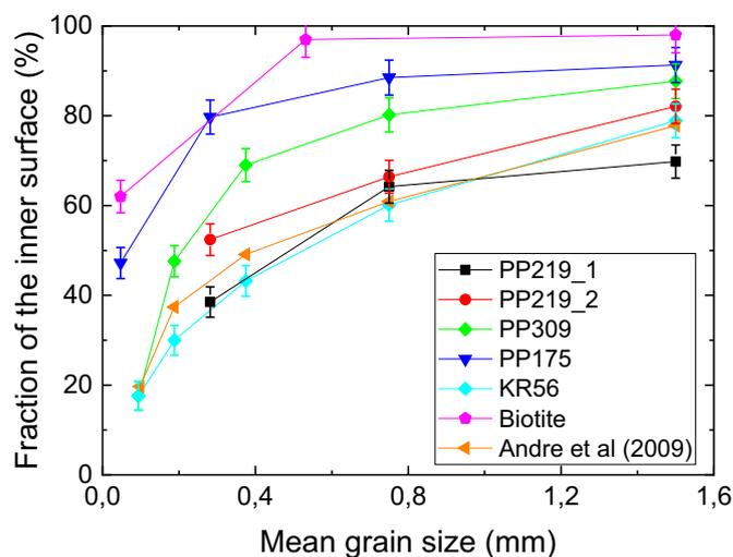
**Fig. 7.** The fraction of inner surface area of the measured specific surface area for different rock samples and biotite as a function of average grain size. The error bars represent the uncertainty of the approach given in 2.3. The results of similar analysis by André et al. (2009b) are also given. Note that the solid lines are used only to connect the data points.
