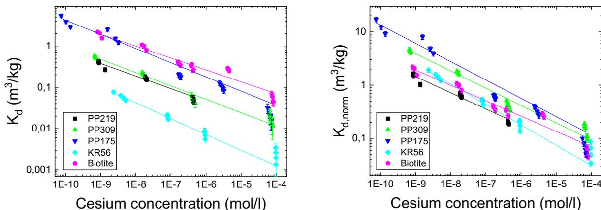
Fig. 1. The distribution coefficient ( $K_d$ ,  $m^3/kg$ ) of Cs on crushed rocks and biotite as a function of equilibrium Cs concentration. The measured distribution coefficients (left) and normalized coefficients ( $K_{d, norm}$ ) according to their mica content (right) are shown. The solid lines show fits by Eq. (7). The error bars are standard deviations of the means of three parallel measurements.
