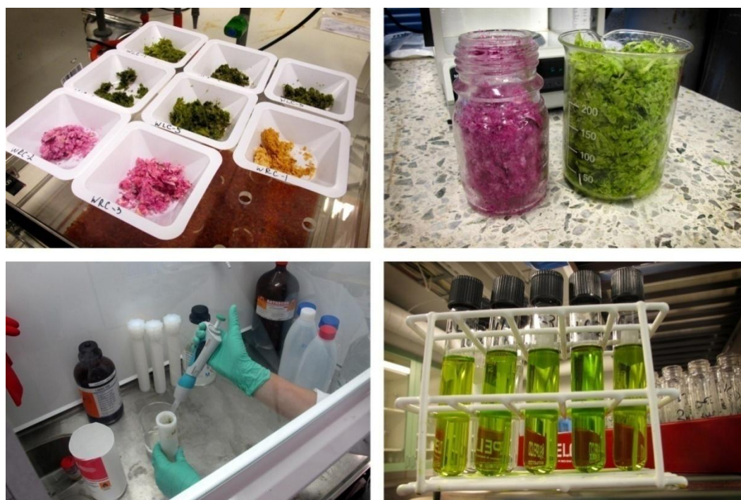
Figure 4. Laboratory analysis procedures. Top left – measuring pretreated crop samples for trace element analysis. Top right – crop samples after they have been disintegrated and freeze-dried. Bottom left – preparing samples for the MARS treatment, as part of trace element analysis. Bottom right – crop sample extract eluted with dichloromethane, as part of the PAH analysis.
