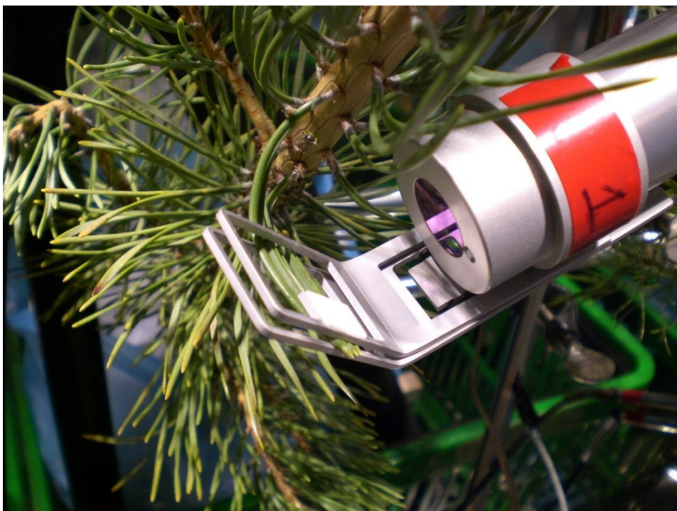
Figure 5. An example of how sensor heads of the monitoring MONI-PAM fluorometer were set to measure the chlorophyll fluorescence signal from Scots pine needles (paper III).
