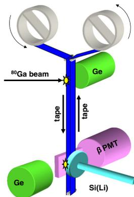
FIG. 1. Schematic view of the experimental setup. The tape moves the collected radioactivity in front of the Si(Li) detector.
