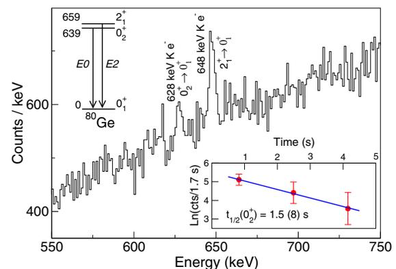
FIG. 2. Energy spectrum obtained from the Si(Li) detector from the decay of  $^{80}\text{Ga}$ . The inset shows the decay curve of the 628 keV  $e^-$ , which is compatible with the  $^{80}\text{Ga}$  lifetime(s). The deduced partial level scheme of  $^{80}\text{Ge}$  is also drawn.
