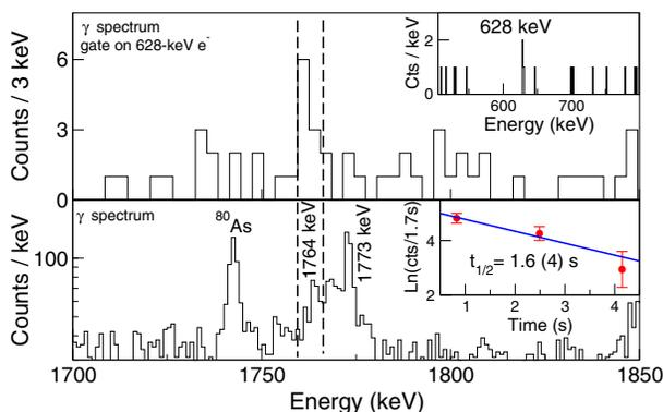
FIG. 3. Upper panel:  $\gamma$  spectrum gated on the 628 keV  $e^-$ . The peak at 1764 keV is clearly visible. The inset shows the inverse coincidence on the Si(Li) spectrum. Lower panel:  $\gamma$  spectrum,  $\beta$  gated, and enlarged in the region of interest. The inset shows the decay curve of the 1764 keV  $\gamma$  ray, compatible with the  $^{80}\text{Ga}$  lifetime(s).
