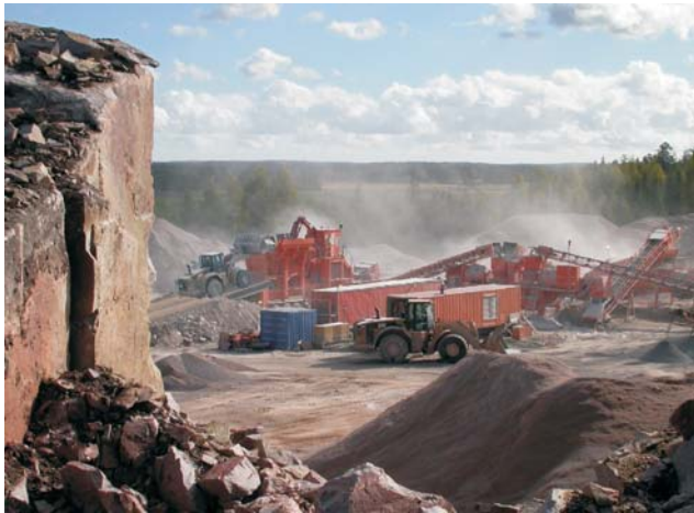
Production of railway ballast and asphalt aggregates in the Pernaja quarry in summer 2004.
