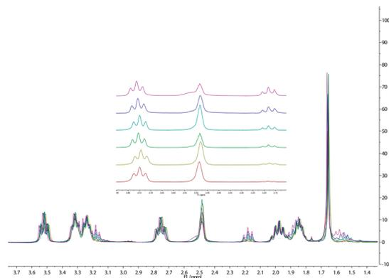
**Fig. 3** Stacked  $^1\text{H}$  NMR spectra of the recycled [DBNH][OAc] showing the hydrolysis product build-up throughout the experiment. Solvent used was DMSO-d<sub>6</sub>. See ESI† for larger image.
