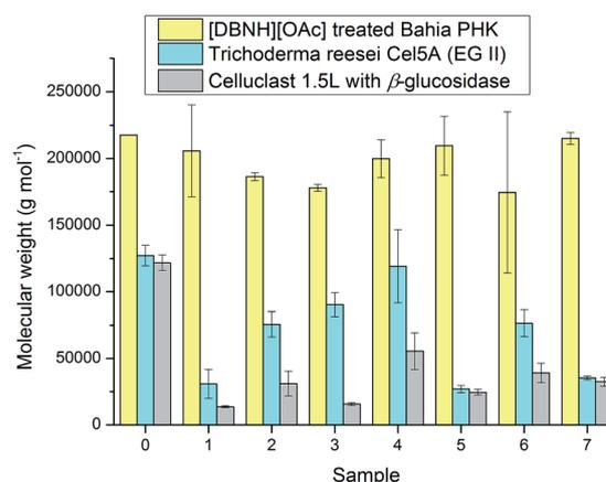
Fig. 8 Weight averaged molecular masses ( $M_w$ ) of enzymatically hydrolysed untreated and [DBNH][OAc]-treated samples. Reference sample  $M_w$ s are in yellow, total hydrolysis (Celluclast 1.5L supplemented with  $\beta$ -glucosidase)  $M_w$ s in grey and partial hydrolysis (*Trichoderma reesei* Cel5A)  $M_w$ s in cyan. The hydrolysis temperature was 45 °C, the time 24 h and the hydrolysis medium 50 mM citrate buffer at pH 5.0.
