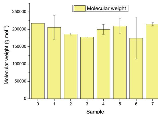
**Fig. 5** Molecular weight values of untreated pulp (0) and pulps treated with recycled [DBNH][OAc] (1–7). Error bars indicate the standard deviation from between two parallel samples.
