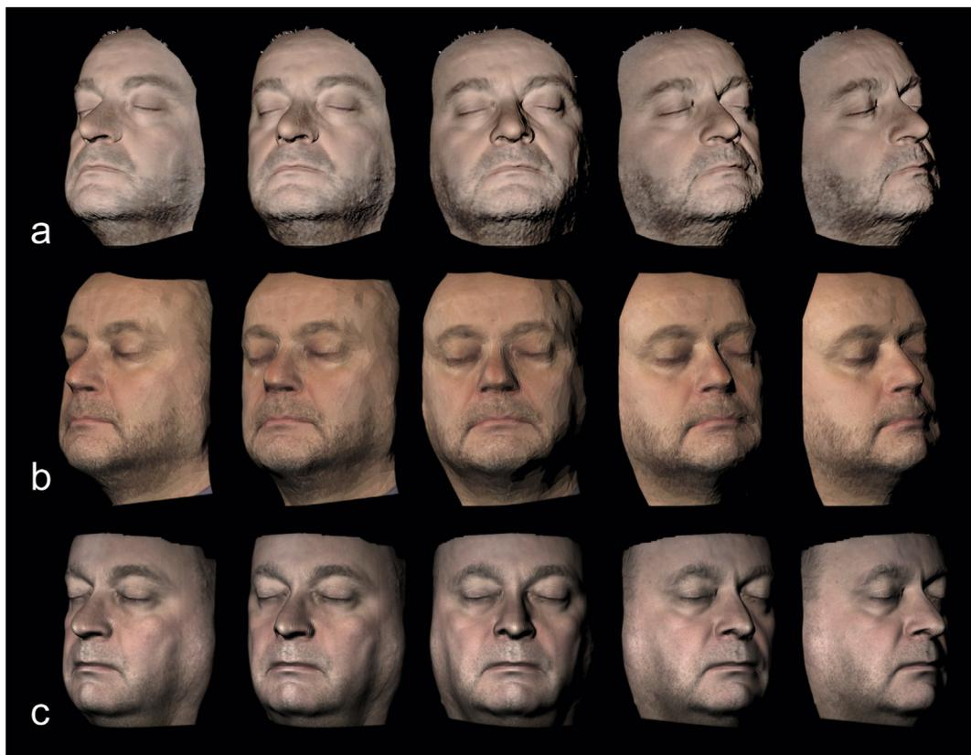
**Figure 1** Three-dimensional (3D) images of the test person using the three techniques: a) DAVID, b) 123D, and c) Proface.
