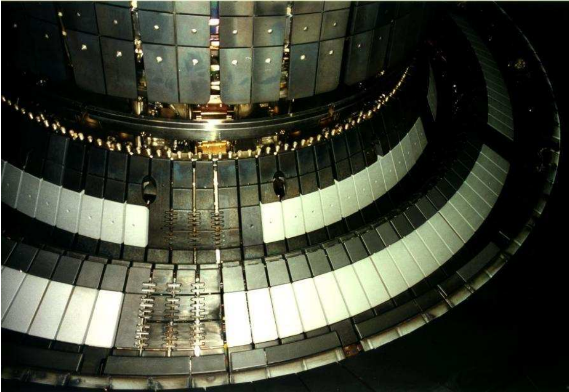
Figure 3: Divertor target plates in the ASDEX (Axially Symmetric Divertor EXperiment) Upgrade tokamak [22], Garching, Germany.
