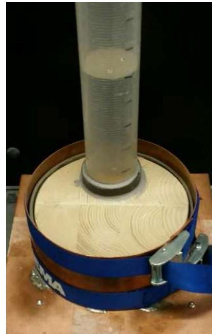
Figure 4: ECT measurements of a wood specimen during water infiltration. ECT Measurement fixture, the wood specimen and the water reservoir mounted on top of the specimen.
