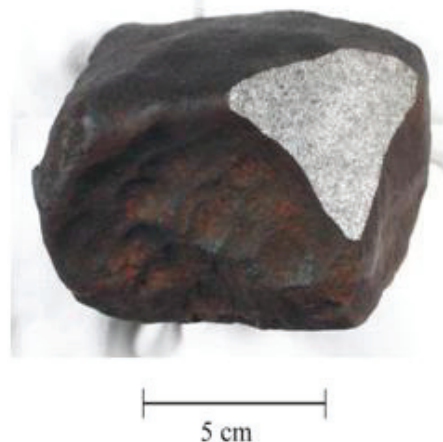
Fig. 1. The Neuschwanstein 1750g fragment found on July 14, 2002. The dark cover is the fusion crust while the fresh interior is exposed on the cut. The samples used in this study are coming from the separated edge.
