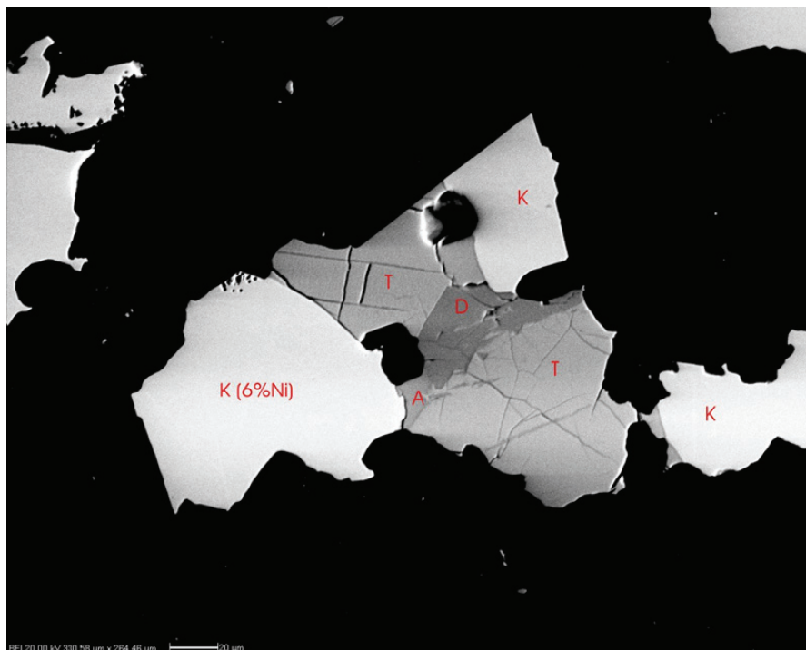
Fig. 5. SEM backscattered electron image of the Neuschwanstein meteorite showing the major metal and sulphide phases. A – alabandite (Fe, Mn)S, D – daubreelite \text{FeCr}_2\text{S}_4 , K – kamacite FeNi, T – troilite FeS. The horizontal dimension of the image is 330.58 \mu\text{m} .
