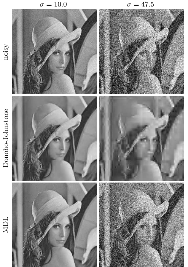
Figure 1: Lena Denoised. Top left : Noisy image ( \sigma = 10.0 ); middle left : Donoho-Johnstone (2.2 % retained, std. error 8.1); bottom left : MDL (7.6 % retained, std. error 6.8); top right : Noisy image ( \sigma = 47.5 ); middle right : Donoho-Johnstone (0.3 % retained, std. error 17.3); bottom right : MDL (46.9 % retained, std.error 44.9).
