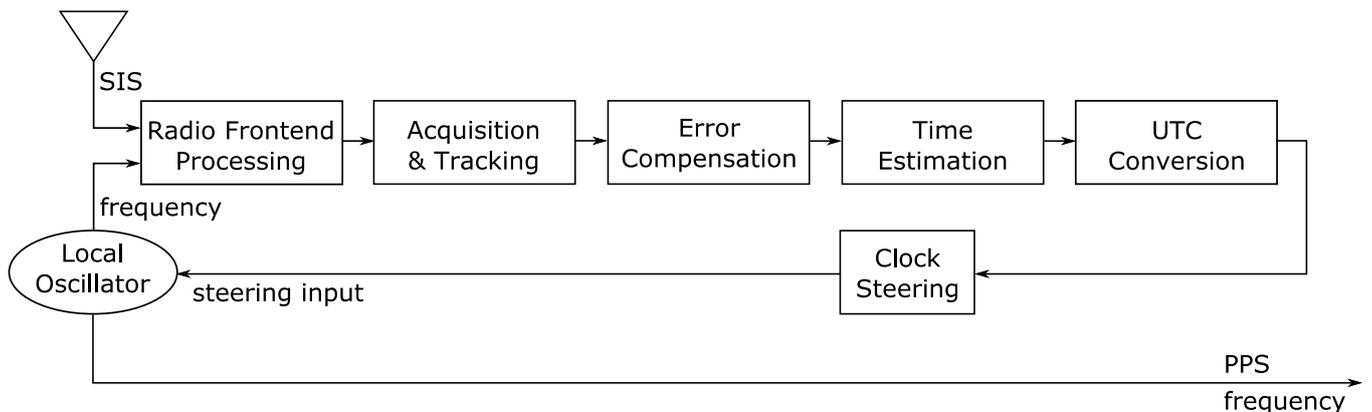
**Figure 2: Basic processing steps for EGNSS based timing.**
