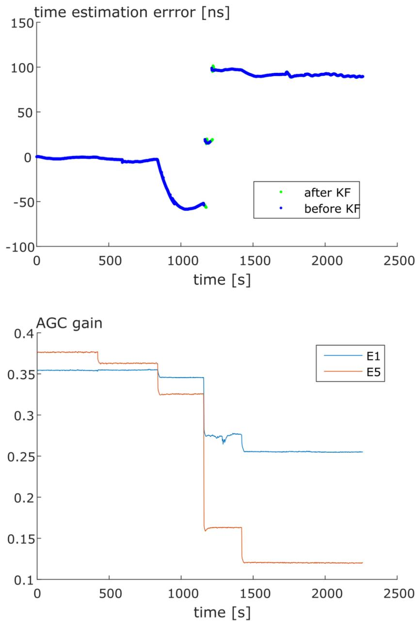
Figure 4: Timing solution (top) and AGC gain (bottom) for a receiver under meaconing.
