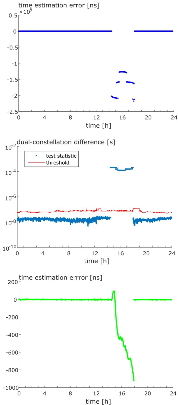
**Figure 6: Application of the dual-constellation cross-check. Top: Galileo timing solution temporarily corrupted when no mitigation is applied; middle: detection statistic from (8); bottom: timing solution mitigated by holdover.**
