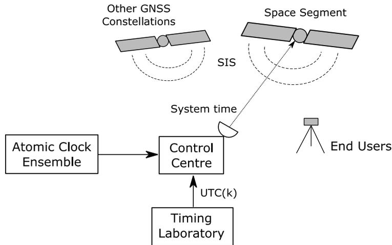
**Figure 1: High-level architecture of EGNSS based timing.**
