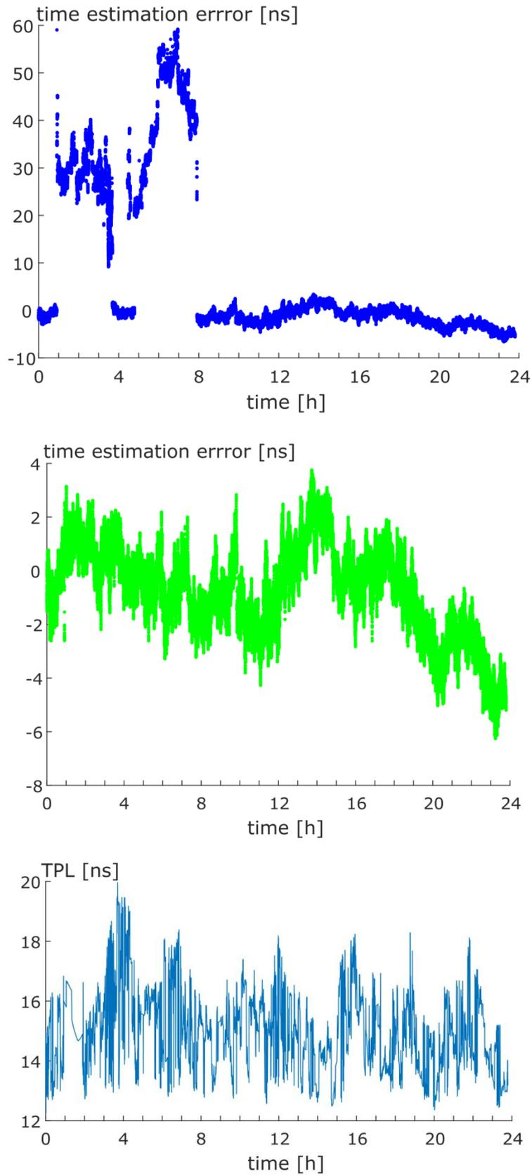
**Figure 5: Effect of T-RAIM. Top: time offset solution without mitigation; middle: time offset with T-RAIM excluding the outlier; bottom: TPL determined with  $p_{FA} = 10^{-5}$  and  $p_{MD} = 10^{-3}$ .**
