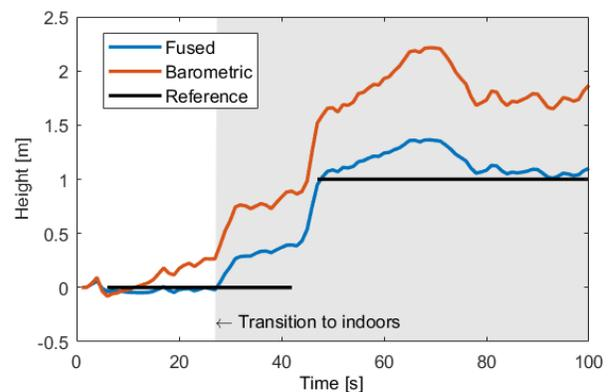
Fig. 13. Detail of Fig. 12 from the first 100 seconds. The transition from outdoors to indoors happens at the line of white and grey area. As the black line indicates, the height should not change but a bias is caused to barometer measurement.
