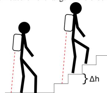
Fig. 2. The average distance measured by sonar (red dotted line) mounted under a backpack increases by  $\Delta h$  when ascending steps. Similarly it decreases when descending steps.
