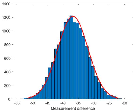
Fig. 4. Histogram of barometer noise obtained by calculating the difference of two barometers measuring side by side in indoor environment. Plotted in red is the normal distribution fitted to data.
