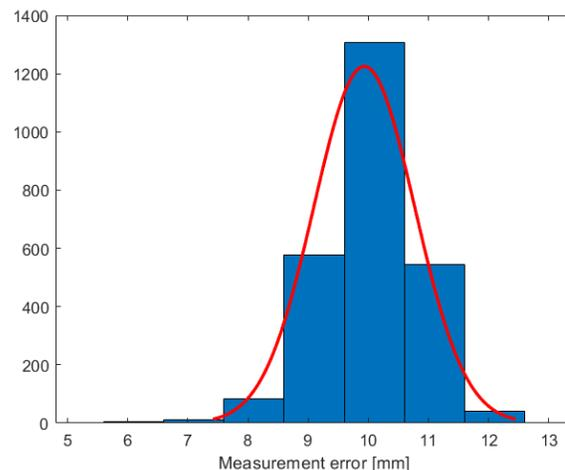
Fig. 5. Histogram of sonar measurement noise obtained by measuring a distance of 1.4 m to a wall in static conditions. Non-zero mean is mainly due to bias in sensor location inside the device.
