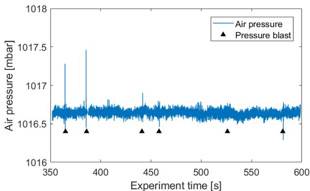
Fig. 9. Pressure measurement during large but short pressure shocks in large open hall area. The blue line plots the pressure and black upward pointing triangles mark the times of pressure shock from a firearm. First and second are measured 5 meters from the source, third and fourth 15 meters from the source and fifth and sixth 4 meters from the source.
