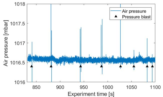
Fig. 11. Pressure measurement during large but short pressure blasts in confined hallway. The blue line plots the pressure and black upward pointing triangles mark the times of pressure blasts from a firearm. In the four first blasts two rounds are fired consecutively. First, second, fifth and sixth are measured 5 meters from the source and the rest 10 meters from the source.
