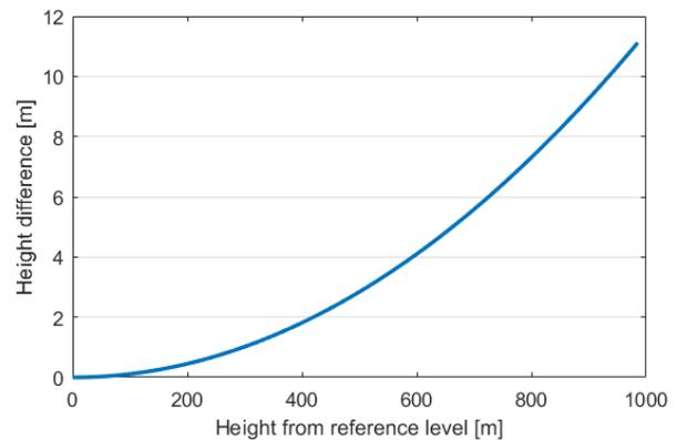
Fig. 1. Height difference of results from equations (3) and (4) at the same pressure height. The horizontal axis is the pressure height from (3) using lapse rate -0.0065 K/m and nominal sea level pressure and temperature.
