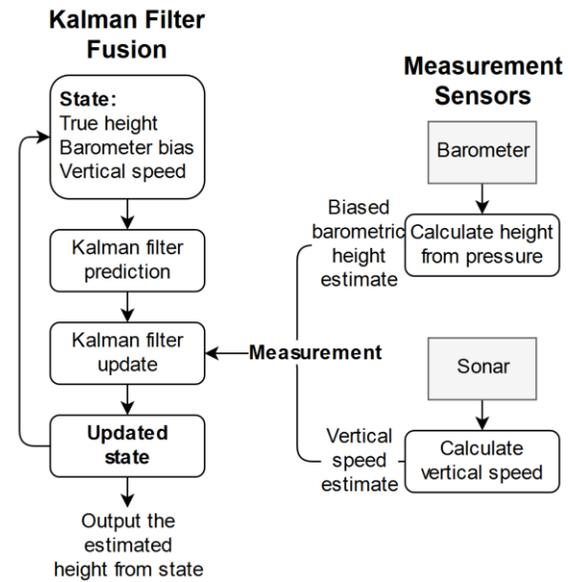
Fig. 3. Flowchart of the presented Kalman filter fusion for height.
