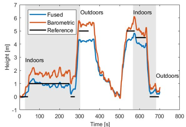
Fig. 12. Barometric height and the Kalman filtered fusion of barometer and sonar compared to reference height track in test number 4. The grey areas mark the time the test person was indoors and the rest of the time the person was outdoors
