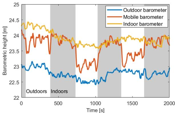
Fig. 6. Barometric height from three different sensors at constant altitude but different environments. Outdoor (white background) and indoor (grey background) areas refer to the location of the mobile barometer.
