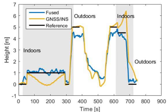
Fig. 14. Comparison of the height solution of barometer-sonar fusion presented in this paper and post processed and smoothed height solution from a commercial tactical grade INS/GNSS system. Both are from test number 3. INS/GNSS solution is obtained with commercial software and is processed both forward and backward and smoothing the end result.
