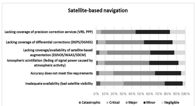
Fig. 5. Significance of lacking coverage and inadequate availability or accuracy of satellite-based navigation and correction services.
