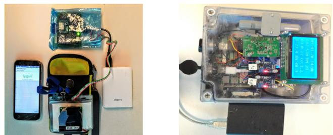
(a) PM<sub>2.5</sub> portable sensor equipped with a GPS, WiFi module and mobile phone connectivity for data logging and visualization [10].
