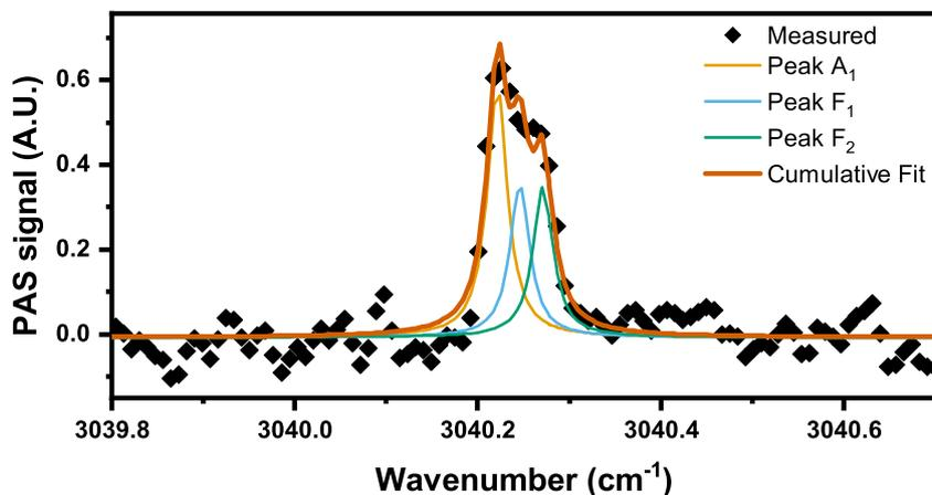
Figure 4: Fit of three Lorentzian peaks on the R(3) line of  $^{14}\text{CH}_4$ . The relative intensities of the three lines were fixed according to the spin statistical weights. Methane R(3) line has one line component of A symmetry and two F components, and each of the two F line components have 3/5 times the area of the A component.
