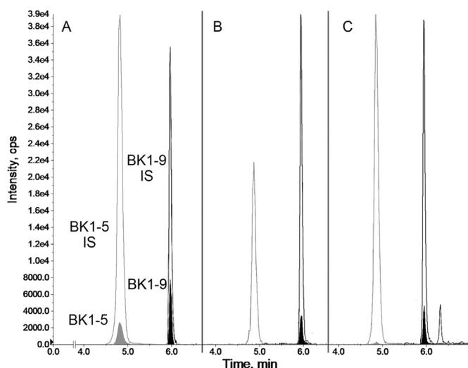
Fig. 2. Chromatograms of bradykinin 1-5 (BK1-5) and bradykinin (BK1-9) calibrator, containing 10 and 1 nmol/l of respective analyte (A), QA sample containing 0.5 nmol/l bradykinin (BK1-9) (B) and a patient sample containing 0.4 nmol/l bradykinin (BK1-9).
