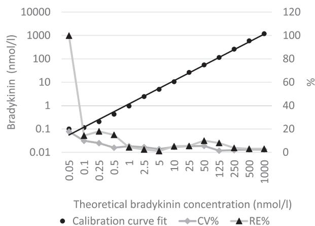
Fig. 3. Linear range ( $R^2 = 0.9959$ ) and accuracy (CV and relative error) of the bradykinin assay.
