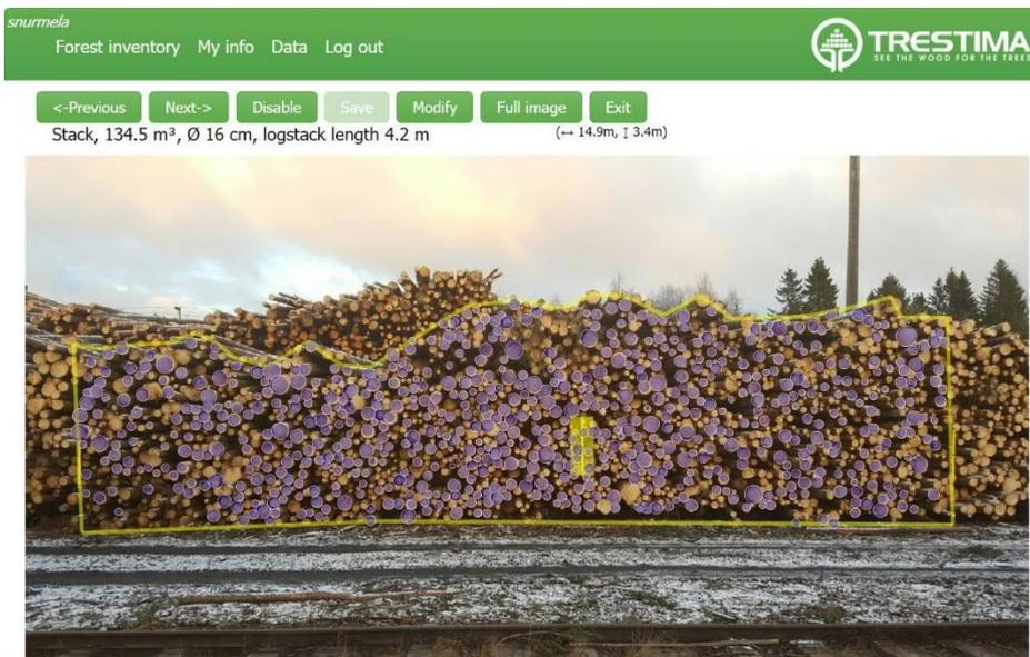
**Fig. 2.** Trestima Stack measurement has been started and three yellow reference sticks of one meter long have been attached to a stack (top). One image from the stack measured has been taken and analysed with the final frame bounded, as well as being checked by Trestima company staff (down).
