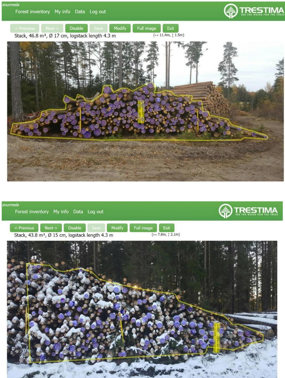
**Fig. 3.** A lot of empty space in the final Trestima image framing around the stack (top) and too tight image framing which leaves logs outside of an image analysis (down).
