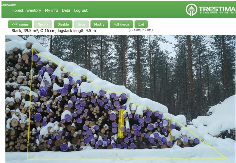
**Fig. 4.** Visual obstacles (e.g. snow cover, tree branches) in the Trestima Stack image cause challenges for the image framing. In this image, a Trestima Stack measurer has estimated that the bottom of stack is under snow cover.
