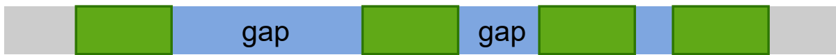
Figure 3.2: An example for gap breaking. Each green block indicates an anchor, and a blue block indicates the BFS connecting path. Depending on the parameters, the first anchor might be ignored due to the large gap between the first and the second anchor.
