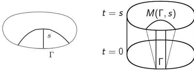
FIGURE 3. The domain of influence of  $\Gamma$  at time  $s$ . The property of the finite propagation speed for the wave equation indicates that when a source function  $f$  is supported on  $\Gamma$  at time  $t = 0$ , then at time  $t = s$  the solution is supported on the domain of influence, that is  $\text{supp}(u^f(s)) \subset M(\Gamma, s)$ .
