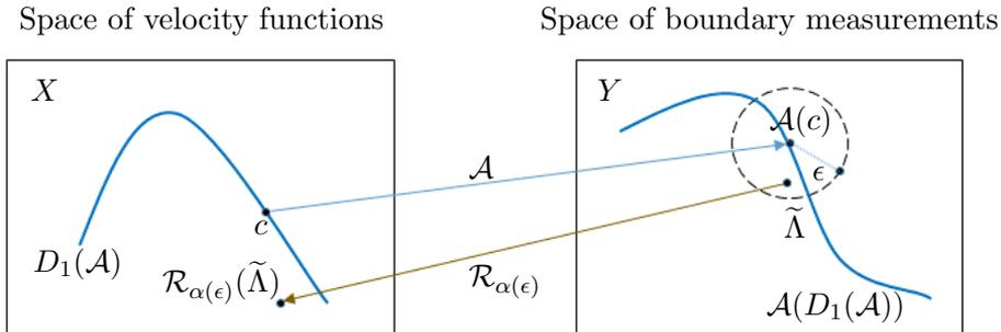
FIGURE 5. The idea of regularization is to construct a family  $\mathcal{R}_{\alpha(\epsilon)}$  of continuous maps from the data space  $Y$  to the model space  $X$  in such a way that  $c$  can be approximately recovered from noisy data  $\tilde{\Lambda}$ . For a smaller noise level  $\epsilon$ , the approximation  $\mathcal{R}_{\alpha(\epsilon)}(\tilde{\Lambda})$  is closer to  $c$ . More details can be found in [64, Fig. 11.5].
