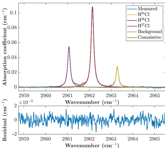
**Fig. 2.** Fit to the measured R(3) lines (upper panel) and the fit residual (lower panel). The three major peaks belong to H<sup>37</sup>Cl (leftmost), H<sup>36</sup>Cl (middle), and H<sup>35</sup>Cl (rightmost). The background fit consists of a constant, a sine function, and two Lorentzian functions for the two small air absorption peaks at approximately 2961.4 cm<sup>-1</sup> and 2961.7 cm<sup>-1</sup>.
