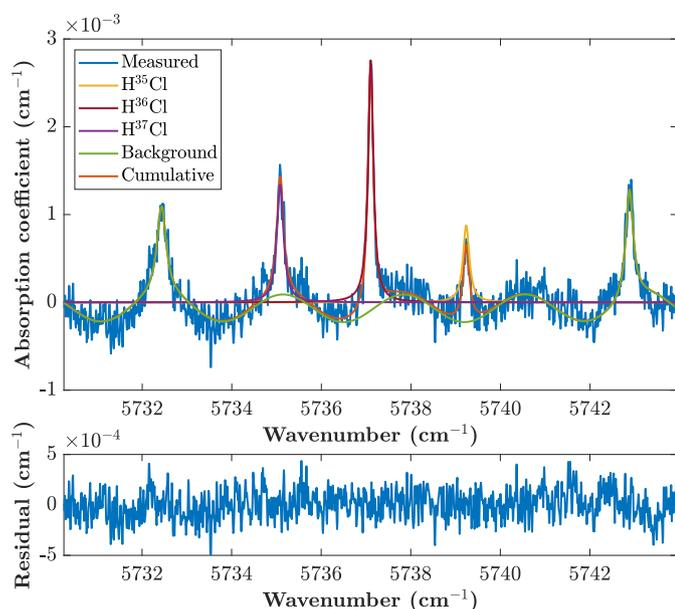
**Fig. 3.** Fit to the measured first overtone R(3) lines (upper panel) and the fit residual (lower panel). The leftmost and rightmost peaks are fitted air absorption lines and the remaining three fitted peaks belong to H<sup>37</sup>Cl, H<sup>36</sup>Cl, and H<sup>35</sup>Cl in the order of increasing wavenumber. In addition to the two air absorption lines, the background function consists of a constant and a sine.
