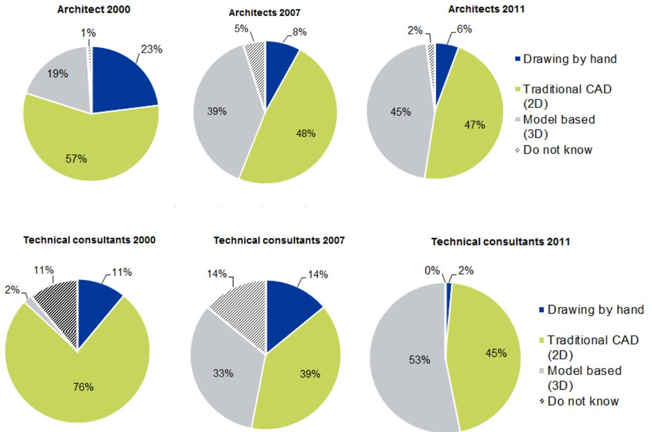
**Figur 3 Proportion of total design time where different tools are used.**
