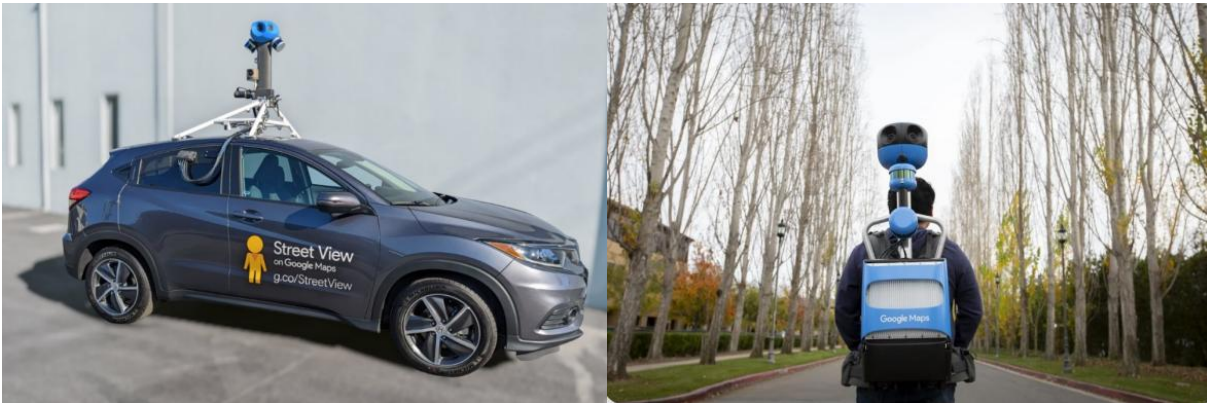
Figure 5. GSV image acquisition methods: (a) Street view car, (b) Trekker
