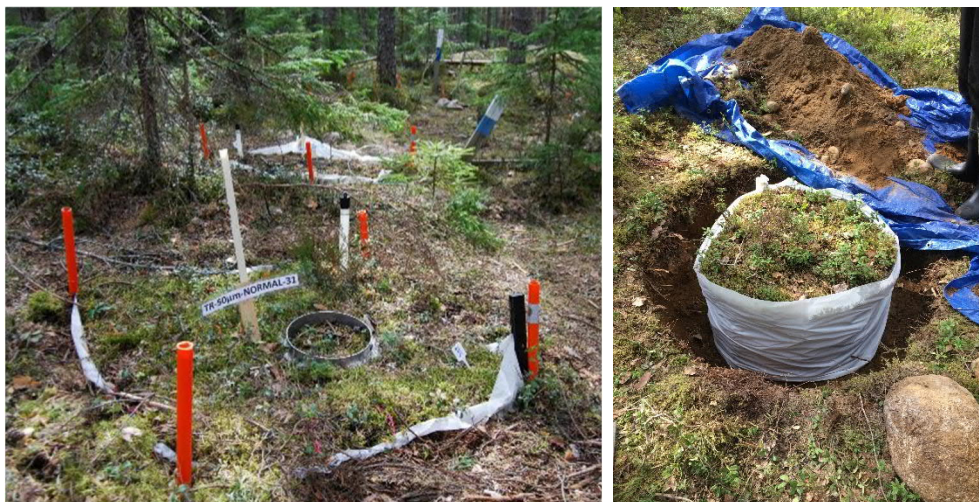
Figure 3. A square root-exclusion (trenching) plot with normal ground vegetation in 2015 (I) (photo by Jussi Heinonsalo) (A), and a round trenching plot under construction after trench excavation and mesh fabric installation around the intact soil in 2017 (III) (photo by Kira Ryhti) (B) in Hyttiälä.
