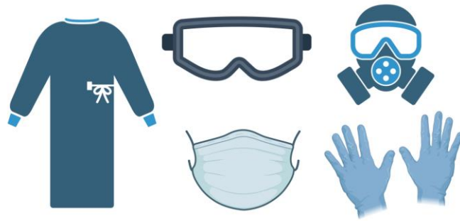
Figure 5. An example of PPEs for a workplace with risk of mercury exposure.
