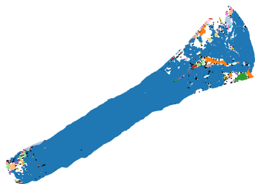
(e) Top view of pc with voxel size 0.01, epsilon 5 and minimum points 10
