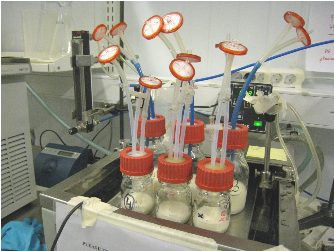
Figure 2. The cold storage system. Raw milk samples were stored for four days in cold (4°C) water bath with continuous stirring and air flow through sterile filters. The original design is by Dr. O. Gursoy, Pamukkale University, Turkey and P. Munsch-Alatossava, Helsinki University, Finland.
