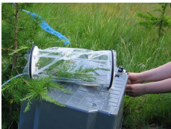
Picture 2. The VOC emission measurements from a Siberian larch with manual flow-through chamber (Paper II).
