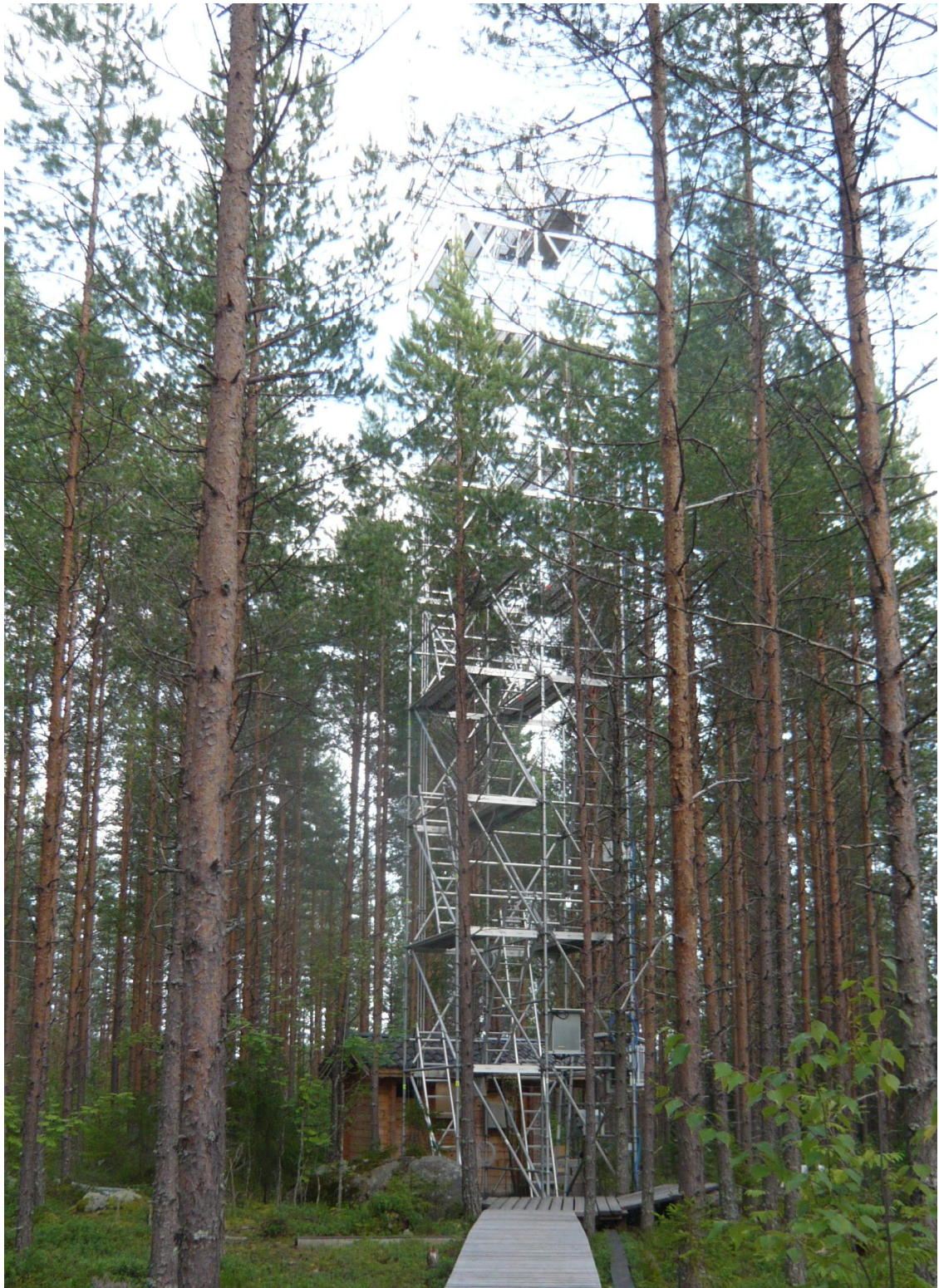
Picture 1. The measurement tower used for the VOC volume mixing-ratio and above-canopy flux measurements at SMEAR II.
