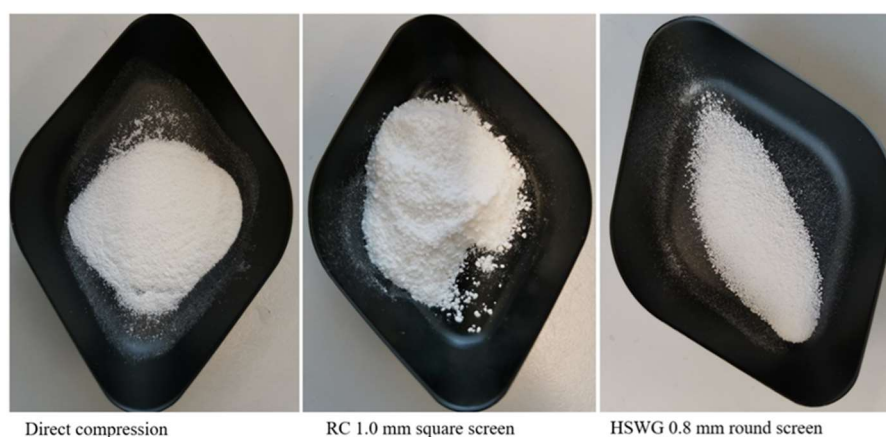
Figure 4. Pictures of direct compression, RC 1.0 mm square screen and HSWG 0.8 mm round screen formulations.
