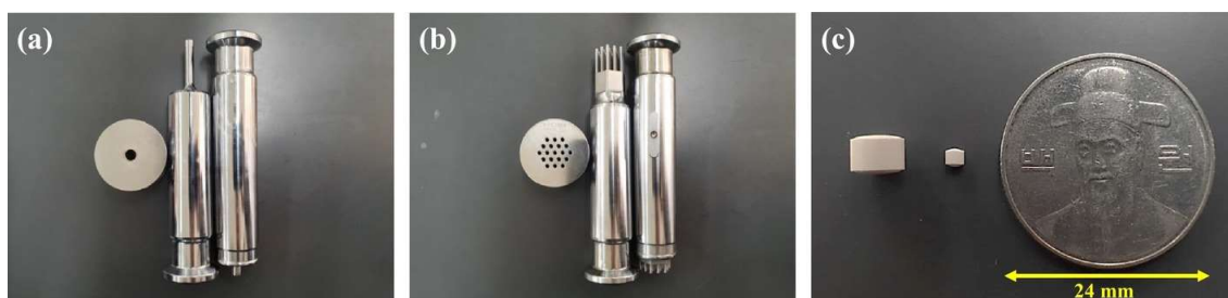
Figure 18. Punches and die for a conventional tablet of 5.5 mm in diameter (a) and multi-tip punches and die used for producing mini-tablets of 2 mm in diameter (b) (Cho et al. 2020). Photo (c) illustrates tablets produced beside a Korean coin (diameter of 24 mm).
