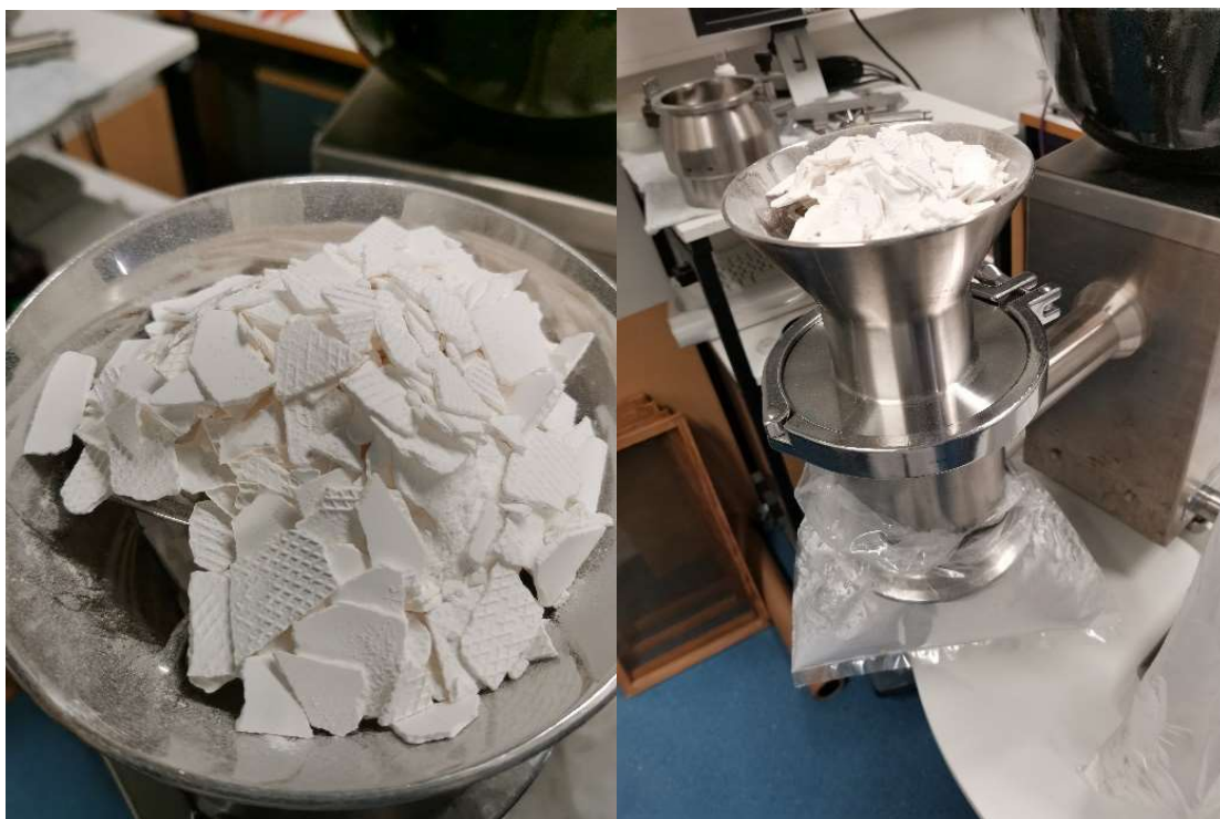
Figure 5. The RC 0.8 mm grater screen milling process in Quadro Comil U5. The fill ratio was high, which might have led to increased residence time and smaller particles.
