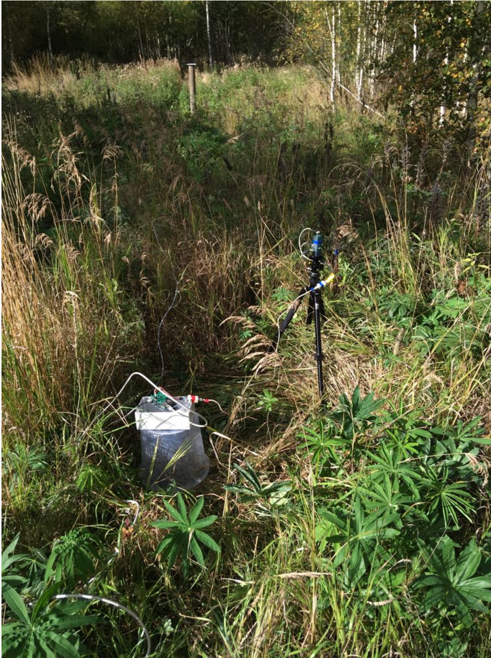
Figure 18: The improved magnetometer being installed at Metsähovi. The magnetometer was mounted on a tripod with a ball head for easy adjustment of orientation. Picture courtesy of Joonas Viuhon.
