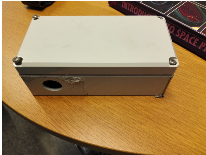
Figure 16: Picture of the magnetometer in its enclosure. The hole on the side was used for passing power and data cables.
