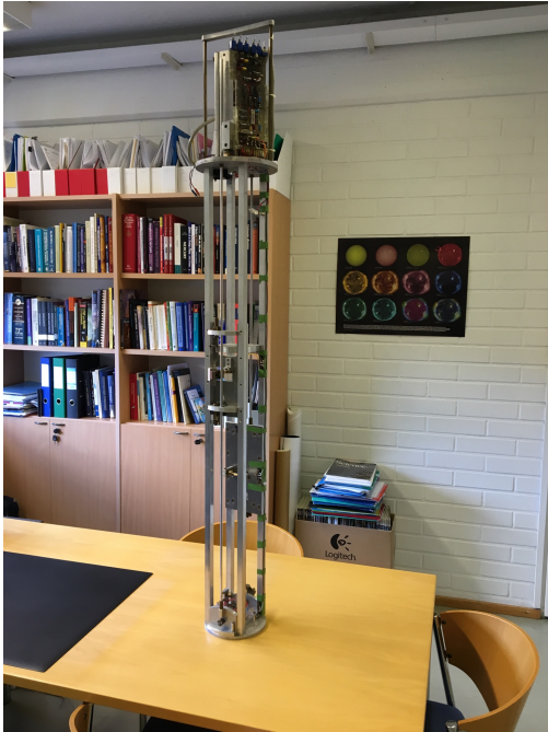
(a) The magnetometer is roughly 1.5 meters tall. The rectangular piece on the top is the light source and camera.
