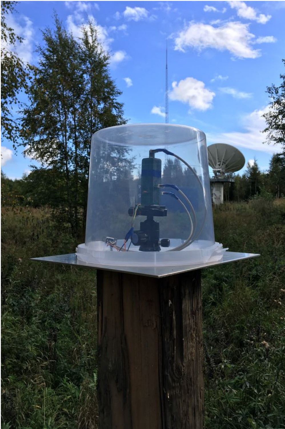
Figure 19: The improved magnetometer with its plastic cover. Picture courtesy of Joonas Viuhko.
