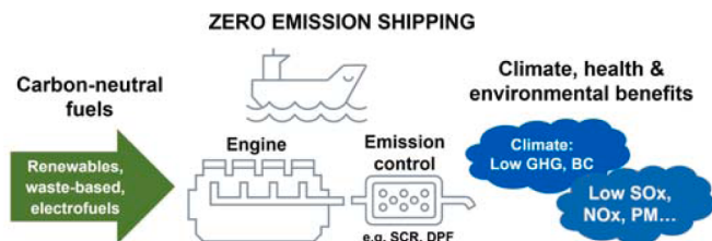
Fig. 1. A combination of carbon-neutral fuels and emission-reduction technologies is needed for (near-to-) zero-emission shipping.
