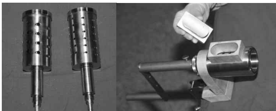
Figure 10: Aesculap bone mills - Left: 6-mm and 3-mm graters. Right: mounted bone mill.
