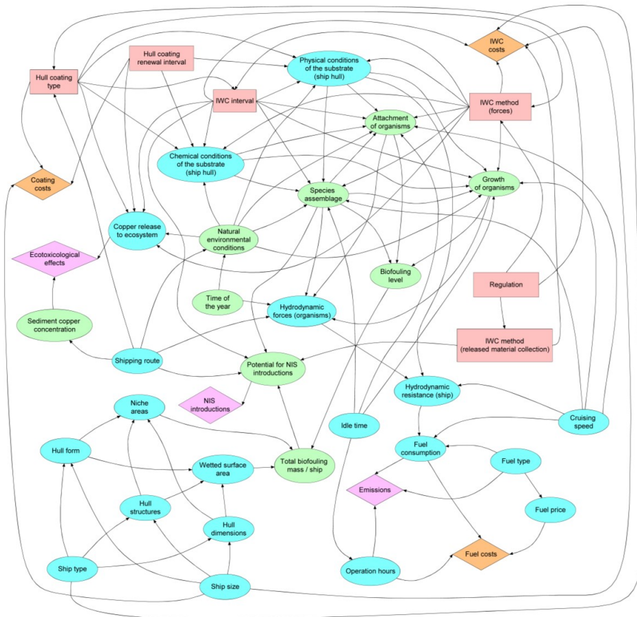
Figure 7. Conceptual influence diagram (CID) of biofouling, from Article IV
