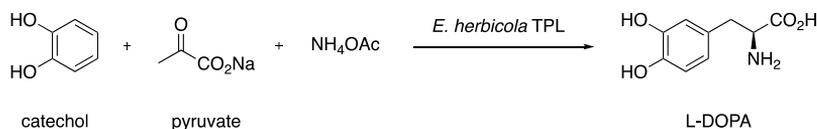
**Scheme 60** Ajinomoto process for the biocatalytic synthesis of L-DOPA.<sup>[186]</sup>
