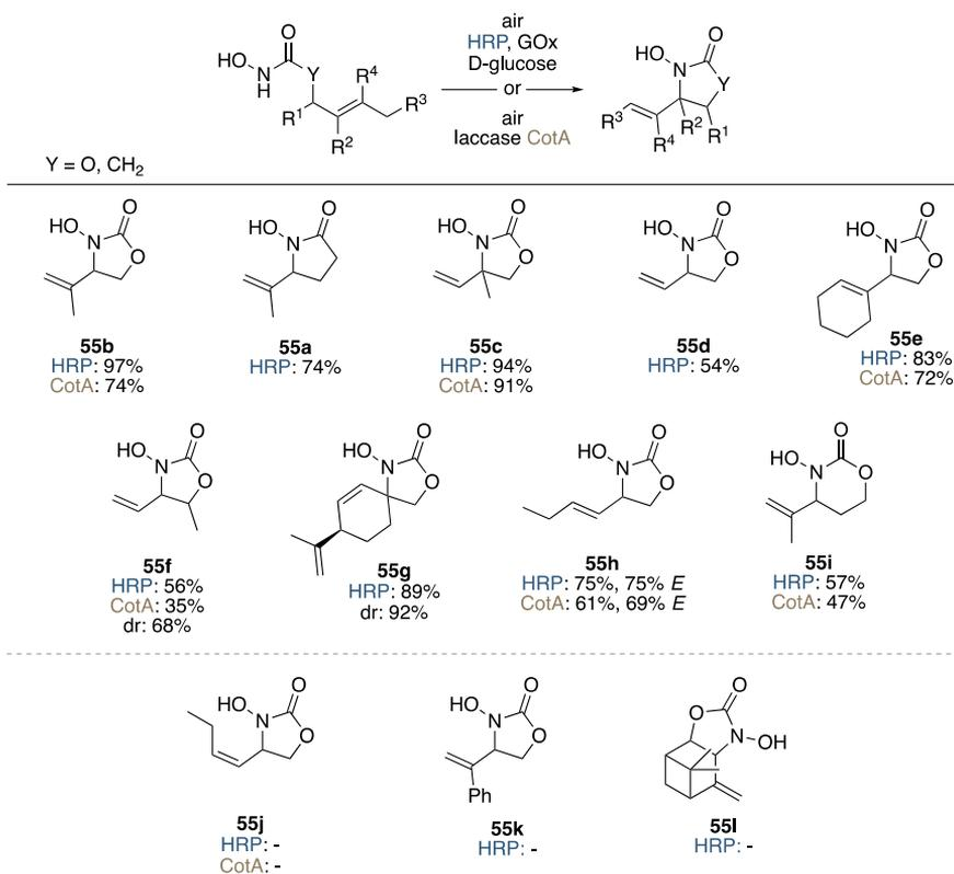
**Scheme 72** Substrate scope of enzymatic nitroso-ene reaction of *N*-hydroxycarbamates.
