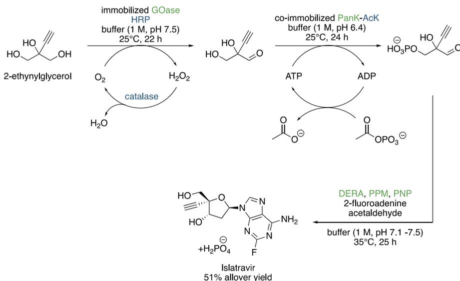
**Scheme 69** Biocatalytic cascade yielding islatravir.
