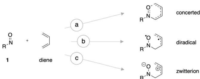
**Scheme 47** Proposed mechanism the NDA reaction of nitroso compounds **1** with a diene.<sup>[148]</sup>
