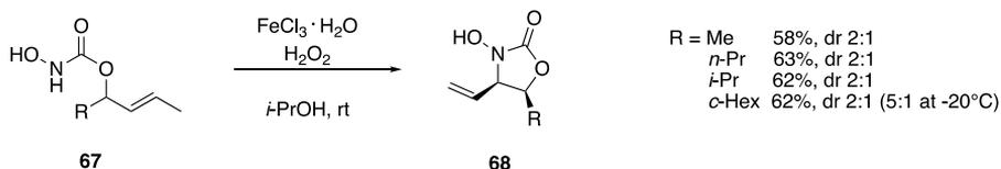
**Scheme 38** Fe-catalyzed oxidation of **67** and in situ intramolecular nitroso-ene reaction leading to diastereoselectivity in the formation of **68**.<sup>[70]</sup>
