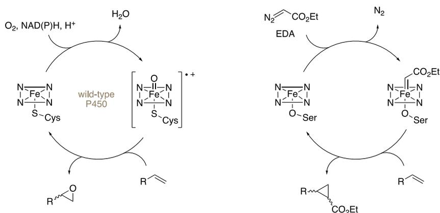
**Scheme 62** Natural epoxidation of olefins (left). Biocatalytic olefin cyclopropanation via carbene transfer (right).
