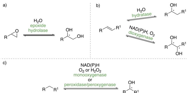
**Scheme 54** Biocatalytic transformations towards alcohols.
