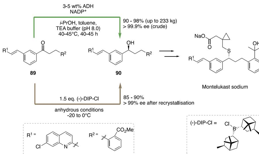
**Scheme 53** Biocatalytic and chemical enantioselective reduction of ketone **89** as a key step in the synthesis of pharmaceutical Montelukast sodium.
