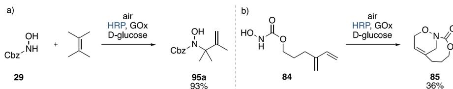
**Scheme 73** a) Biocatalytic intermolecular nitroso-ene reaction. b) Biocatalytic intramolecular NDA reaction.
