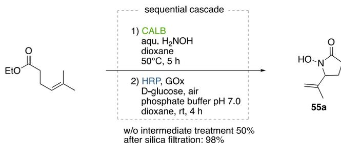
**Scheme 79** Sequential cascade of the hydroxylaminolysis and nitroso-ene protocol.
