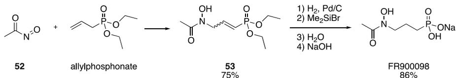
**Scheme 32** Synthesis of antimalarial drug FR900098 via the nitroso-ene reaction of nitrosocarbonyl methane **52** and diethyl allylphosphonate.<sup>[113]</sup>
