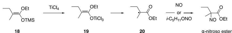
**Scheme 12** Nitrosation sequence yielding  $\alpha$ -nitroso esters using external NO sources.
