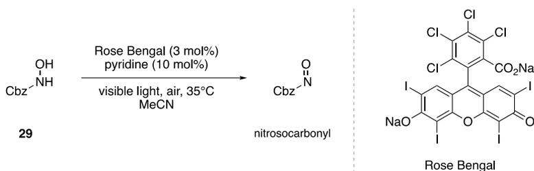
**Scheme 17** Photocatalyzed formation of the nitrosocarbonyl using Rose Bengal.
