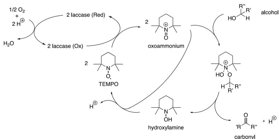
**Scheme 68** Proposed mechanism of alcohol oxidation catalyzed by laccase/TEMPO.<sup>[219]</sup>
