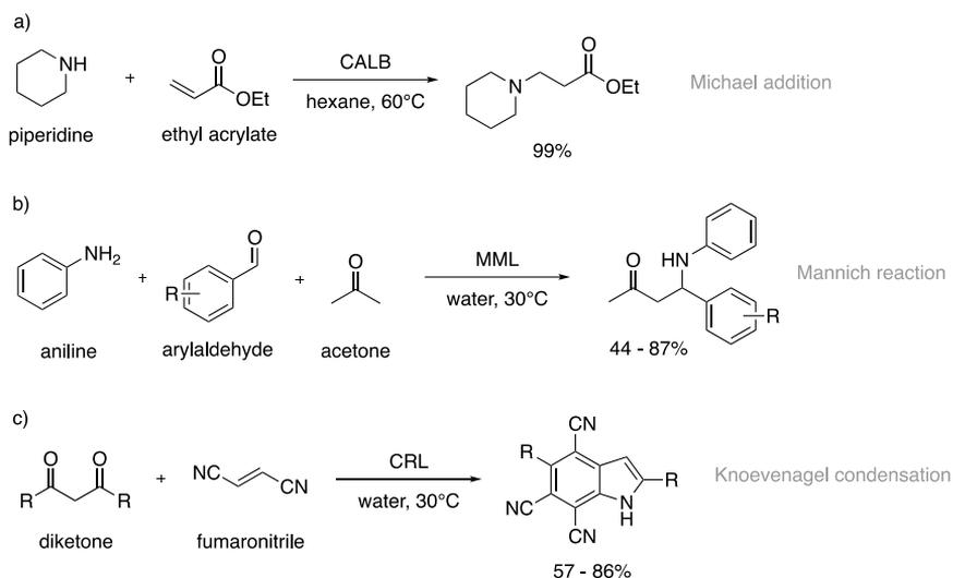
**Scheme 59** Example of biocatalytic transformations towards amines utilizing lipases.<sup>[187–189]</sup>
