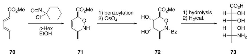
**Scheme 40** Diels-Alder reaction of diene **70** and  $\alpha$ -chloronitroso cyclohexane leading to amino acid **73**.
