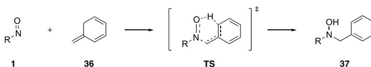
**Scheme 24** Proposed concerted mechanism of nitroso compound **1** and *o*-isotoluene **36**.<sup>[99]</sup>
