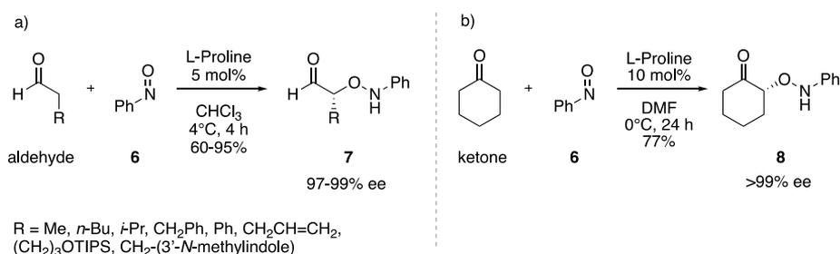
**Scheme 4** Enantioselective  $\alpha$ -aminoxylation of a) aldehydes<sup>[27]</sup> and b) ketones<sup>[28]</sup> with catalytic L-proline.
