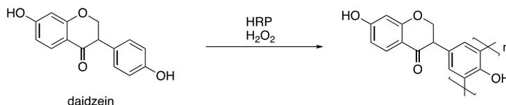
**Scheme 64** Polymerization using horseradish peroxidase (HRP).
