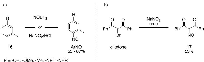
**Scheme 11** Nitrosation via a) aromatic substitution<sup>[55]</sup> and b) halogen-NO exchange<sup>[56]</sup> using external NO sources.
