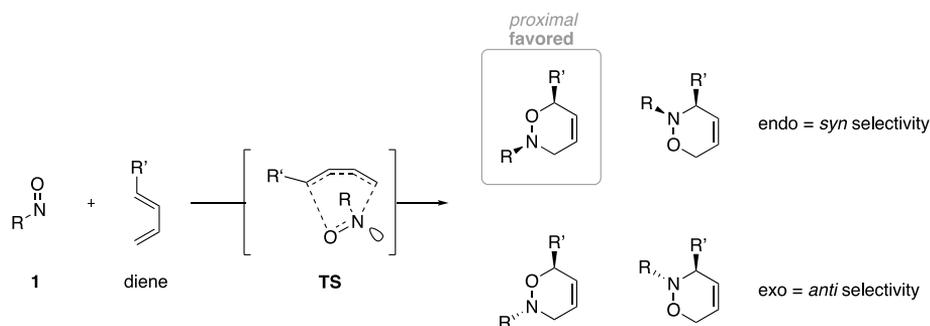
**Scheme 48** Proposed mechanism for the NDA reaction with normal electron demand.
