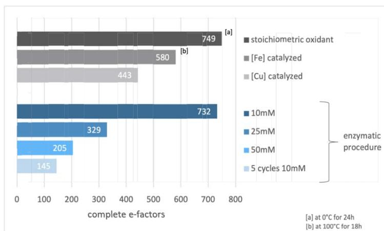
**Figure 10** *E*-factor analysis of the nitroso-ene reaction. Extraction solvents were not taken into account.
