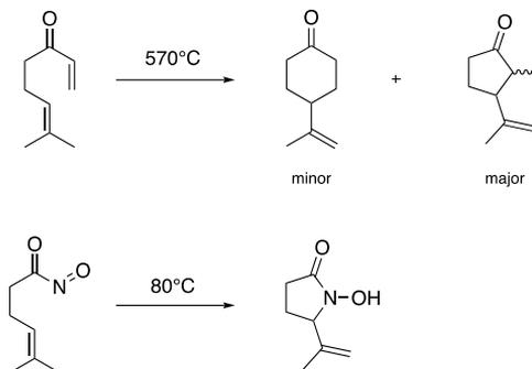
**Scheme 19** Thermal ene reactions of enophiles bearing different reactivity.<sup>[7,91]</sup>
