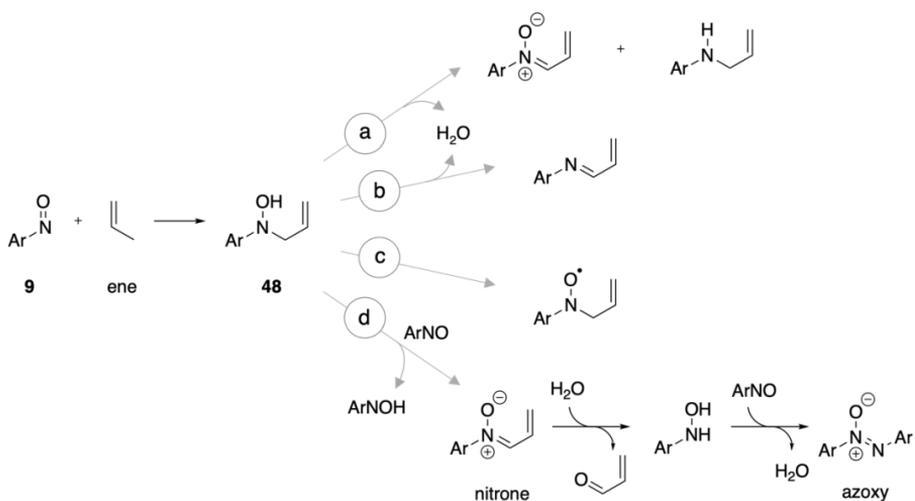
**Scheme 29** Degradation pathways of the ene adduct **48** derived from the nitroso-ene reaction of **9** with an olefin as ene.<sup>[20]</sup>
