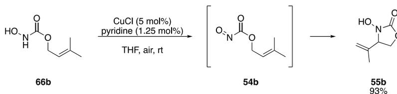
**Scheme 37** Cu-catalyzed oxidation of **66b** and intramolecular nitroso-ene reaction of **54b**.<sup>[71]</sup>
