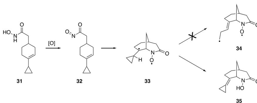
**Scheme 23** Nitroso-ene reaction of **32** following a diradical pathway without opening of the cyclopropyl ring.<sup>[98]</sup>
