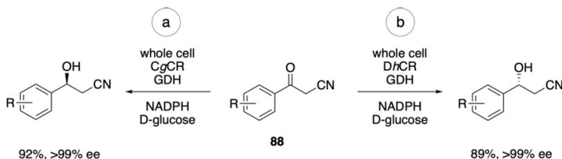
**Scheme 52** Stereocomplementary bioreduction of ketonitrile **88**.<sup>[169]</sup>
