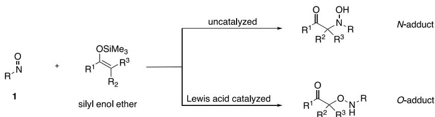
**Scheme 3** Regiocontrol in the nitroso-Aldol reaction utilizing silyl enol ethers.<sup>[21]</sup>
