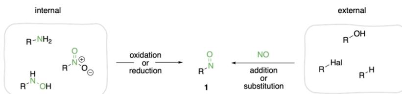
**Scheme 10** Formation of nitroso compounds **1** using internal and external NO sources.
