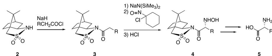
**Scheme 2** Auxiliary-controlled diastereoselective nitroso-Aldol reaction utilizing Oppolzer's sultam **2**.<sup>[10]</sup>
