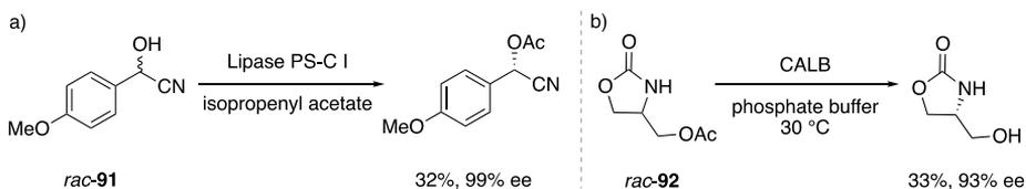
**Scheme 55** Kinetic resolution of alcohol *rac*-**91** and acetate *rac*-**92** using lipase in different conditions.<sup>[178,179]</sup>
