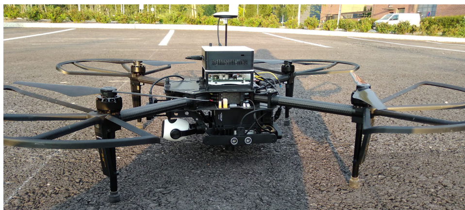
FIGURE 8 | DJI Matrice 100 drone equipped with a Zenmuse Z3 RGB camera. [Color figure can be viewed at wileyonlinelibrary.com ]
