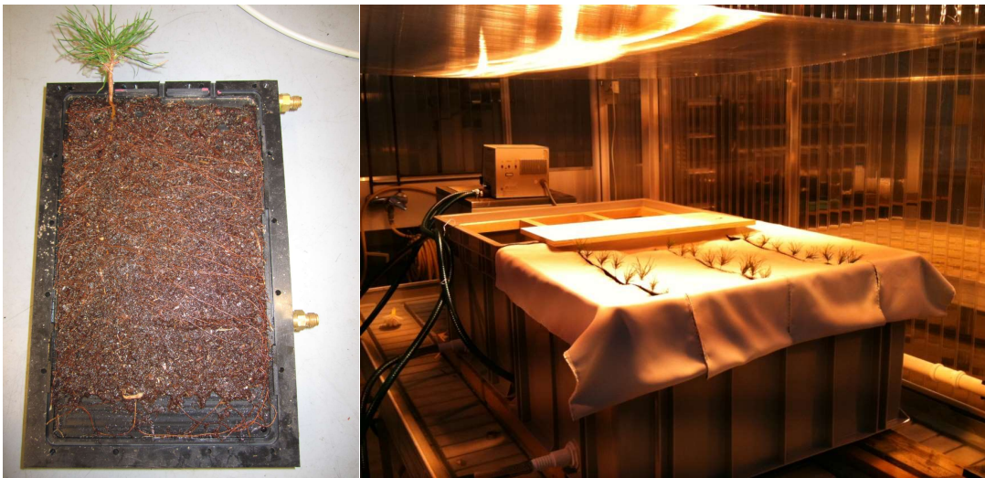
Figure 4. Example of a microcosm system with peat and a pine seedling (left) and setup for the microcosm systems in a greenhouse with the Lauda cooling system (right). Photos: Maiju Linkosalmi
