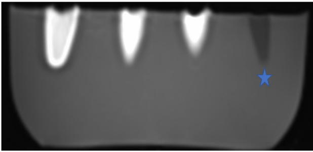
Fig. 3 MRI (3 Tesla) of gadolinium-containing immunoliposomes at different concentrations in vitro with T1 sequence seen as white area in phantom, and control (tap water) seen as grey (star)
