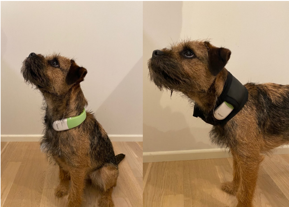
Figure 3 The neckband device without (left) and with the protective cover (right). Images reproduced from studies I and II (supportive material). Photographs: Iida Niinikoski.
