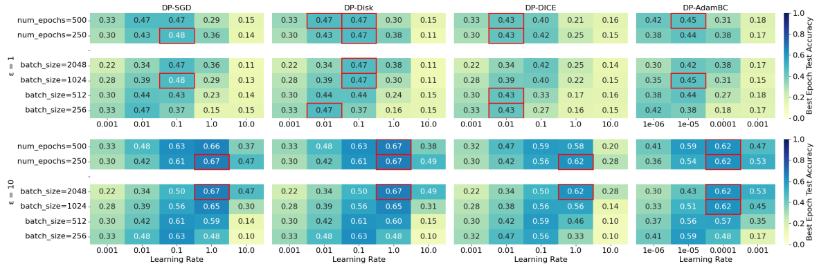
Figure 5.4: Setup 1: Heatmaps showing the best test accuracy for each optimizer on the CIFAR-10 problem, across learning rates (x-axis) and either batch size or number of epochs (y-axis), at \epsilon = 1 (top row) and \epsilon = 10 (bottom row). Each cell reports the best accuracy found over all other hyperparameters. Red boxes mark the highest accuracy per optimizer. DP-SGD consistently achieves the best results, followed by DP-DiSK, then DP-AdamBC, with DP-Dice performing worst.
