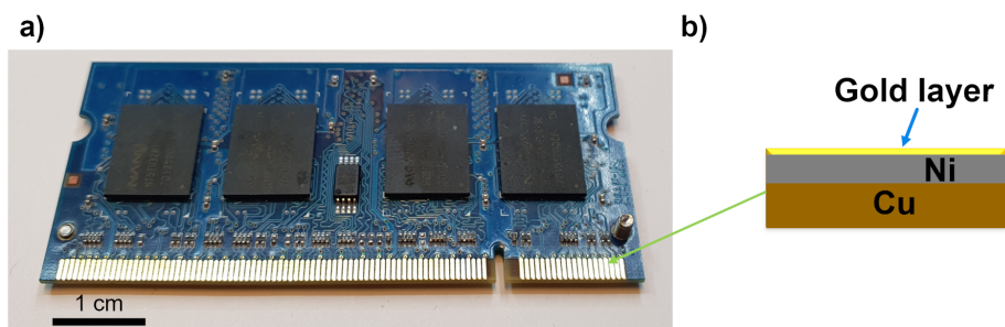
Figure 1 a) A discarded PCB with gold connectors. b) Schematic of the structure of a single gold pad (cross-section, not to scale). The thin gold layer is typically 1–2 \mu\text{m} thick and the nickel layer beneath 3–6 \mu\text{m} thick.
