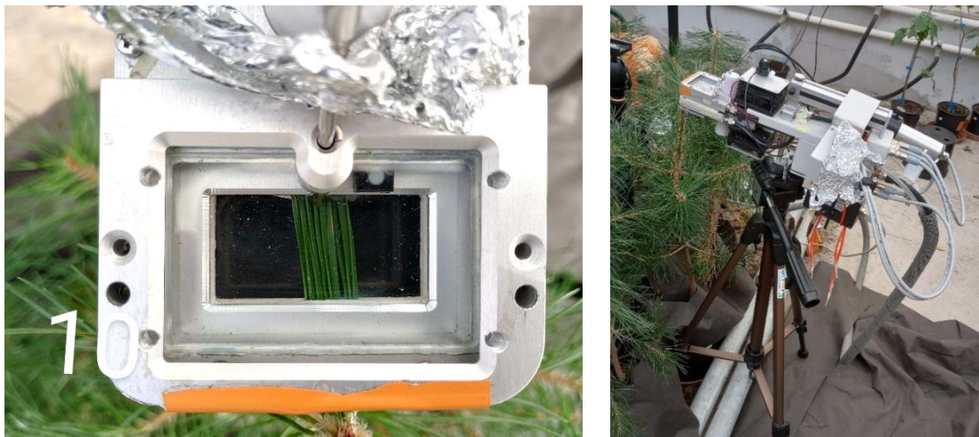
Figure A3. GFS3000 measuring head cuvette with needles inside (left) and the whole setup (right).
