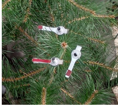
Figure A2. Three open dark-adaptation clips on the primary shoot of a sample plant.
