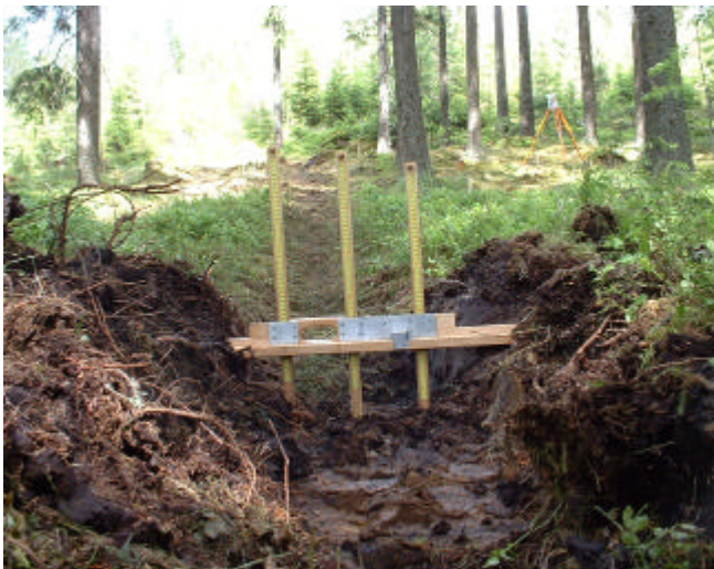
Figure 5.1. Measuring of the rut depth
