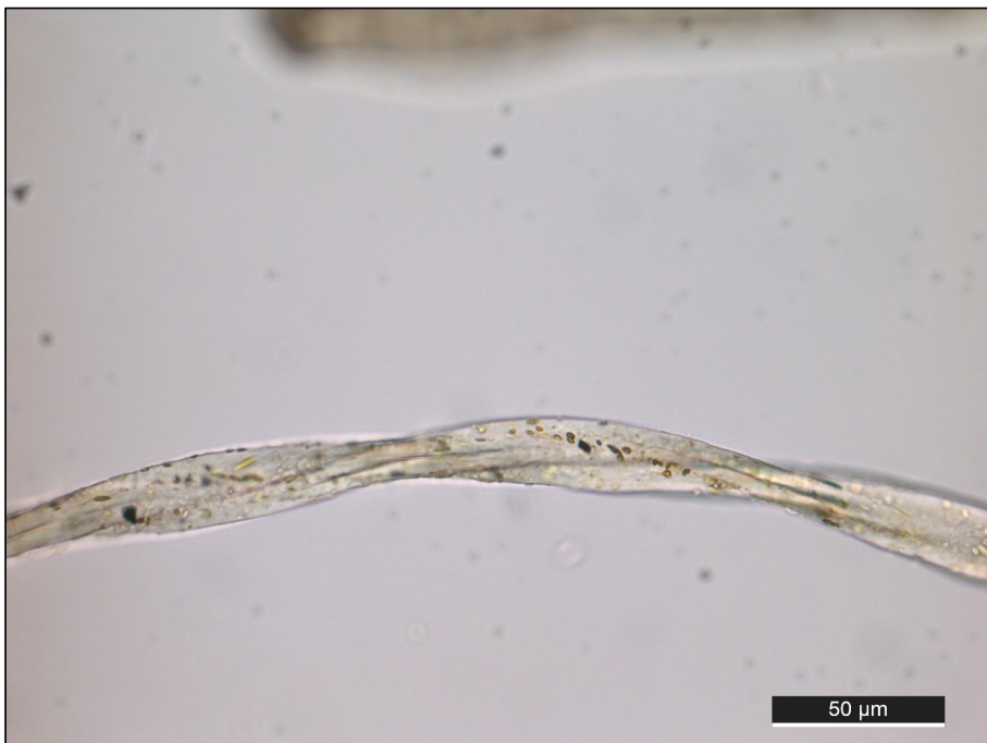
Figure 13 Mould spores on the cotton fibre from the tying ribbon of otsipanta (SU4522:81).
