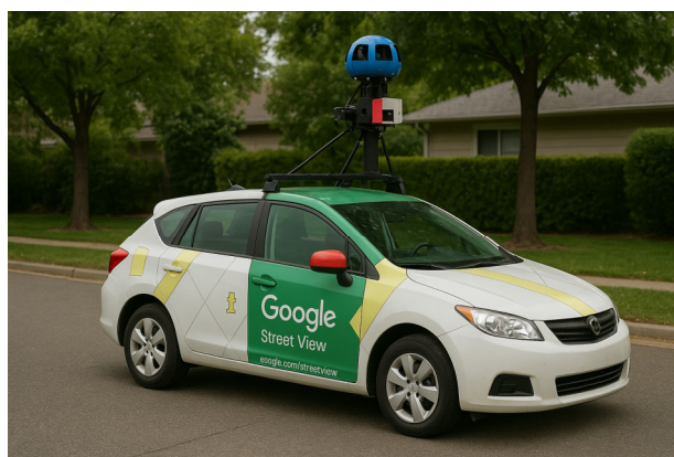
Figure 1. A mobile mapping system was developed by Google to be mounted on a car. The customized LiDAR configurations in Google’s car show how the system is designed for collecting suitable data for 360 virtual tour web-portal.
