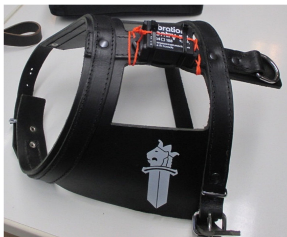
Figure 3. Three-dimensional accelerometer attached to dogs' harnesses.
