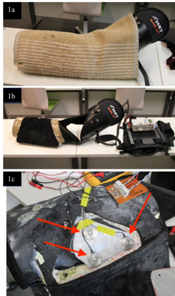
Figure 1. (1a) Left-hand bite sleeve with embedded measurement equipment. (1b) The bite sleeve without the surface material. (1c) Three force sensors (indicated by arrows) fitted into the deepest layer of the bite sleeves.
