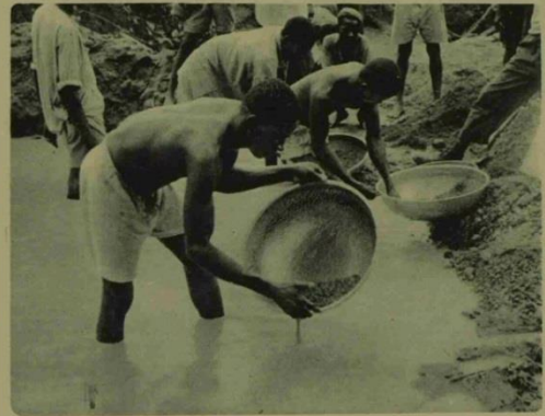
WORKING WITH LARGE SIEVES: DIGGERS PANNING THE DIAMONDFEROUS SOIL. AFTER A BAD HARVEST IN 1952 THERE WAS A RUSH OF ILLICIT DIGGING.
