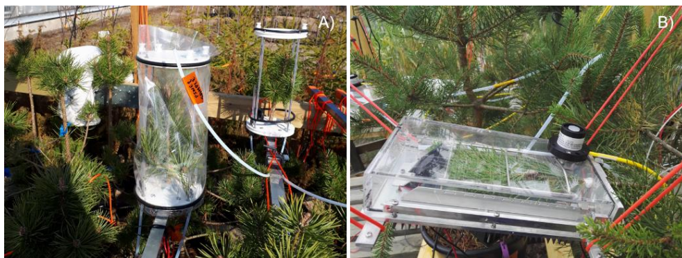
Figure 1. Manual (A) and automated (B) shoot chambers used in the greenhouse gas flux measurements. In (B), the PAR sensor is placed onto the lid of the measurement chamber.
