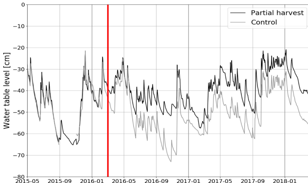
Fig. 3. Daily mean water table level in the control (grey) and harvest site (black line) averaged over all the forest transect measurement points (4, 8, 12 and 22.5 m from the ditch) from May 2015 to April 2018. The harvesting (red vertical line) was carried out in February-March 2016. (For interpretation of the references to color in this figure legend, the reader is referred to the web version of this article.)
