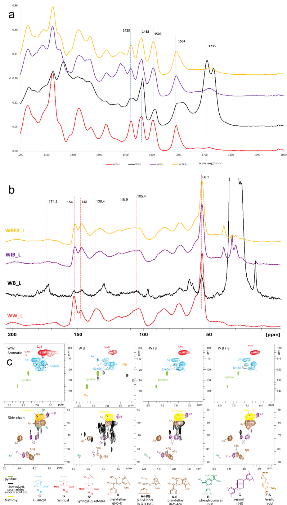
Fig. 5 Chemical characteristics of the dioxane lignin (L) from WW, WB, WIB, and WBF. (a) FT-IR spectra. (b) CP-MAS ^{13}\text{C} NMR spectra. (c) 2D HSQC NMR spectra (DMSO- d_6 /pyridine- d_5 , v/v 4/1) showing the aromatic ( \delta\text{C}/\delta\text{H} , 96–150/6.0–8.2 ppm) and side-chain ( \delta\text{C}/\delta\text{H} , 48–92/2.0–6.0 ppm) regions. See ESI Tables 11 and 12 † for the assignments.
