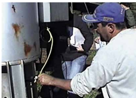
Figure 7.12 Farmer showing the cause in the loose ignitor of the combustion system
